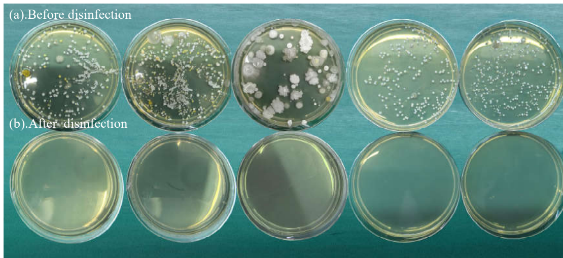
Figure 5: Comparison of Bacterial Colonies in Petri-dishes: Before and After Disinfection.
